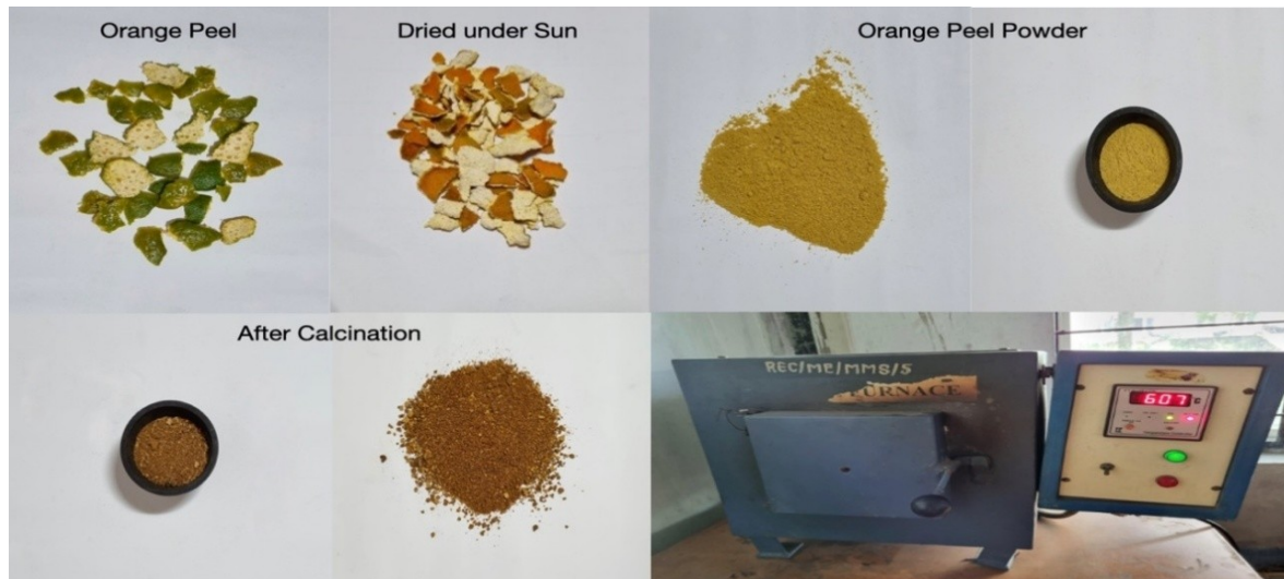
Figure 1. Stages of calcination for orange peel extract.
